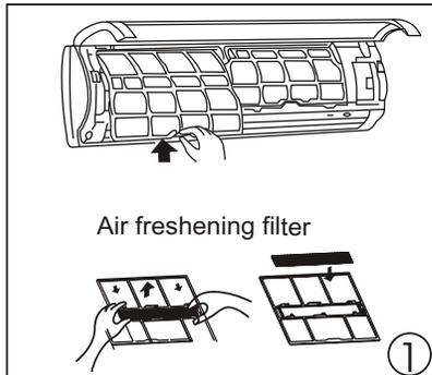
4. Remove the Air Freshening Filters from supporting frame (The solution to disassemble may differ from each other for different filters. Refer to ① and ② ). Clean the air freshening filter at least once a month, and replace it every 4-5 months.
